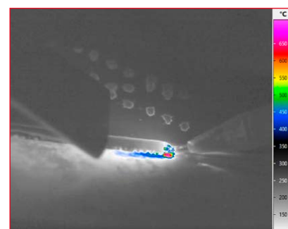
Thermal analysis during laser soldering
